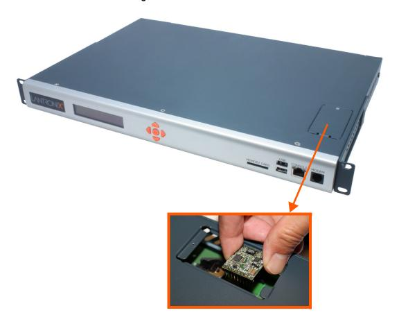
Figure 2-9 Internal Modem Location
